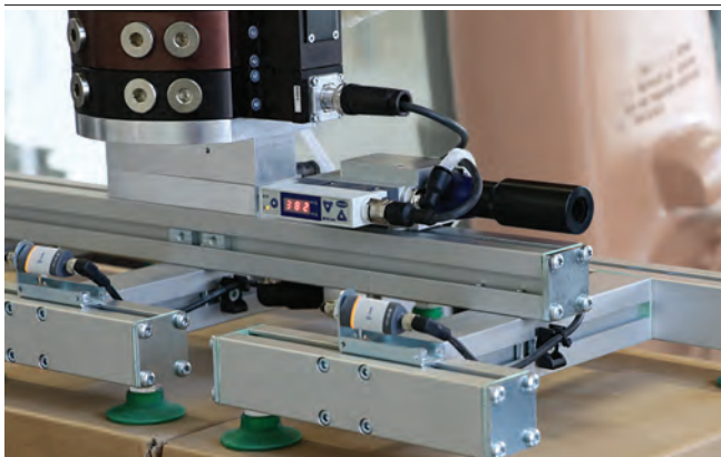
Central vacuum generation by compact ejector SCPSi-L
