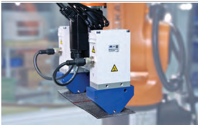
Needle grippers SNGi-AE being used for handling composite textiles
