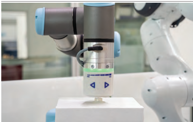
Flat suction cups SUF for handling cardboard boxes
