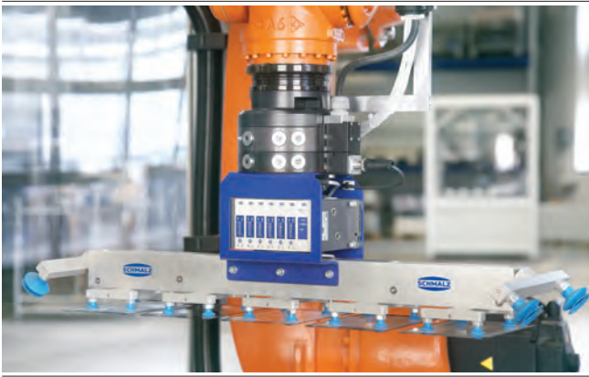
Compact Terminal SCTSi IO-Link handling display glass
