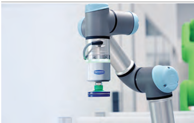
Electrical vacuum generator ECBPMi for handling cans
