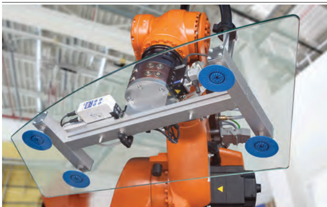
Central vacuum generation by compact ejectors X-Pump SXPi / SXMPi
