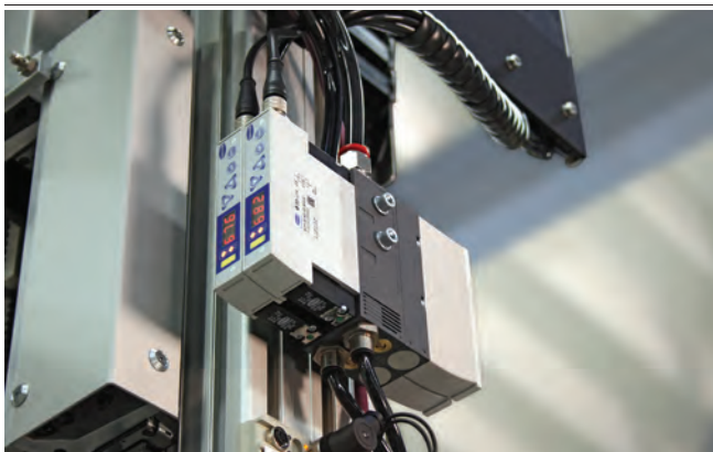
Centralized vacuum generation by compact ejectors SMPi
