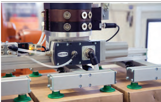
Central vacuum generation with basic ejectors SBPL
