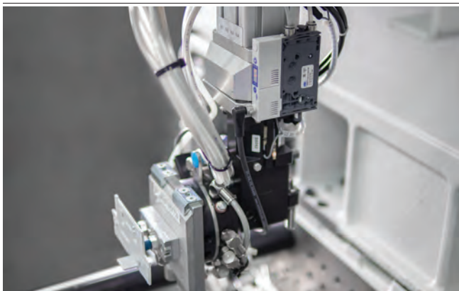
Compact ejector SCPMc handling a plastic part
